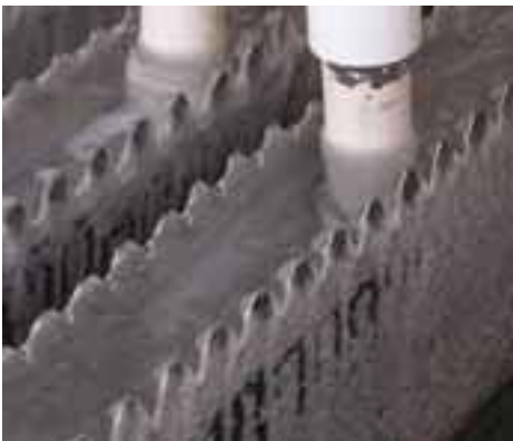
Initial hard deposits on plate ice machine forms within a few days, has to be cleaned with acid.
