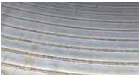
Initial hard deposits on rotary ice machine forms within a few days.
